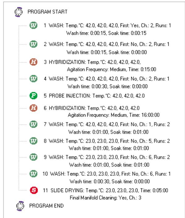
The protocol outlined above has been optimized for hybridization of fluorescently labeled cDNA (transcriptional profiling) and genomic DNA (comparative genomic hybridization) to arrays of cDNA and long oligonucleotides, using the Corning® Pronto!™ Universal Hybridization Kit. The protocol includes steps for both prehybridization and hybridization.
